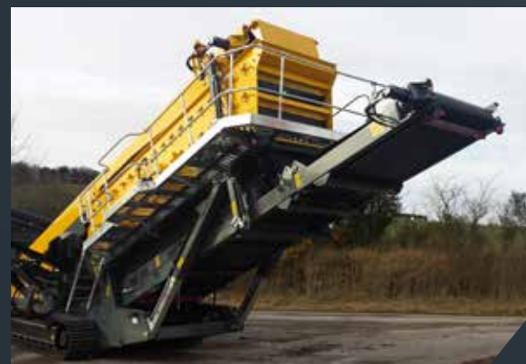
High power screenbox Features adjustable inclination and achieves exceptional results with an amplitude of up to 10 mm and the highest capacity even with difficult materials.
