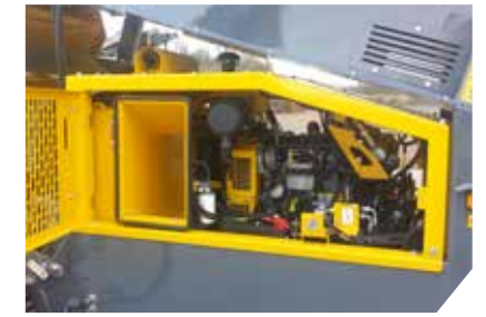
Wide access engine compartment doors Provide perfect access for service and maintenance of engine and hydraulics.
