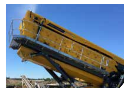
Rinser option Wet screening for increased product quality.
