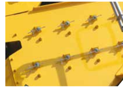
Wedge clamping system Rapid and user-friendly screen change.
