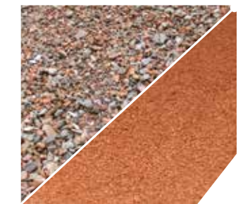
Screened C&D waste fractions
